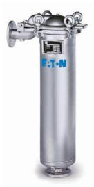
**TOPLINE** single bag filter housing is simply the best from its high-performance design to its investmentcast components. The top inlet design requires less headroom and directs liquid flow through the cover which improves sealing, reduces product loss and makes filter bag change-outs cleaner. ASME coded.
